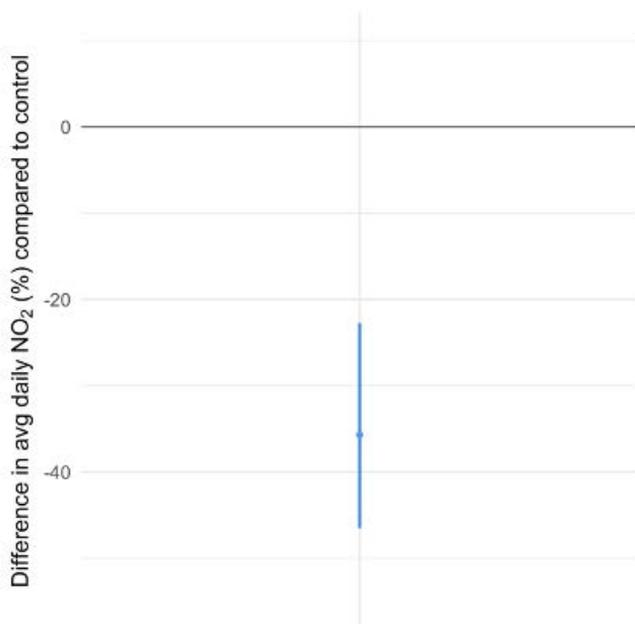
**Figure B1.** Effect of the induction stove intervention on daily average NO<sub>2</sub> exposure in a 24-hour period. Post intervention NO<sub>2</sub> levels were 35.7% lower (indicated with the dot) in kitchens with induction stoves compared to those with the gas stoves after adjusting for outdoor temperature, apartment level, and street orientation. 95% confidence intervals were -46.5 to -22.7% (indicated with the error bars).
