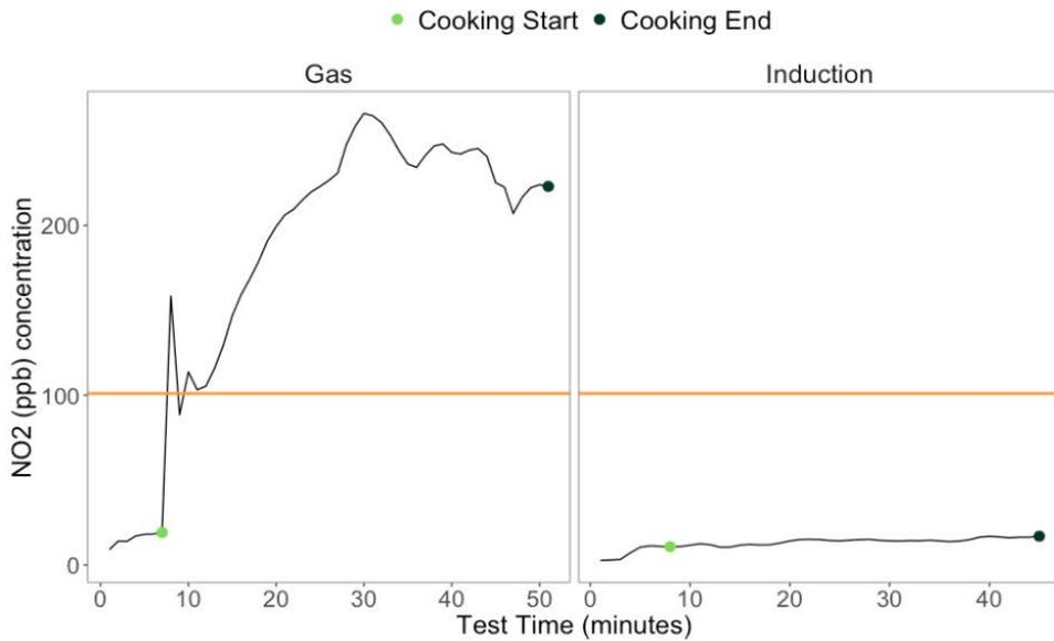
**Figure 2:** Real time NO<sub>2</sub> (ppb) concentrations during controlled cooking events with a gas and induction stove, respectively. The start of the cooking is noted with a light green dot and the end noted with the dark green dot. The orange horizontal line (101 ppb) indicates the EPA threshold for one-hour NO<sub>2</sub> averages that are considered “Unhealthy for Sensitive Groups.”
