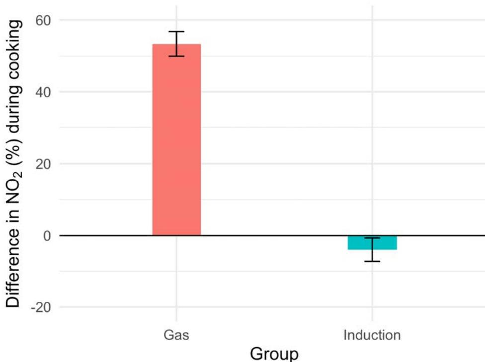
**Figure 3:** Estimates of the effect of the intervention on NO<sub>2</sub> levels during cooking. NO<sub>2</sub> levels increase by 53.3 percent (95% CI: 50.0, 56.8%) during cooking for people using a gas stove, but only a negligible difference in NO<sub>2</sub> levels (-4.0%, 95% CI: -7.3%, -0.7%) is observed during cooking for people cooking with an induction stove. Point estimates (dots) and confidence intervals (error bars) are derived from Model 2.
