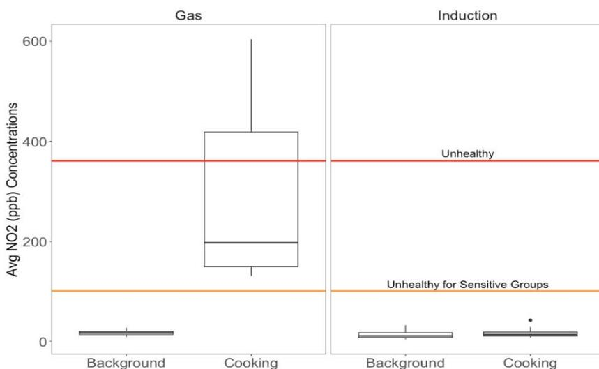
**Figure 1:** Boxplot of mean NO<sub>2</sub> concentrations during gas and induction stove cooking tests compared to the background NO<sub>2</sub>. The orange horizontal line (101 ppb) indicates the EPA threshold for one-hour NO<sub>2</sub> averages that are considered "Unhealthy for Sensitive Groups." The red horizontal line (361 ppb) indicates the EPA threshold for one-hour NO<sub>2</sub> averages that are considered "Unhealthy" for all individuals.<sup>46</sup>
