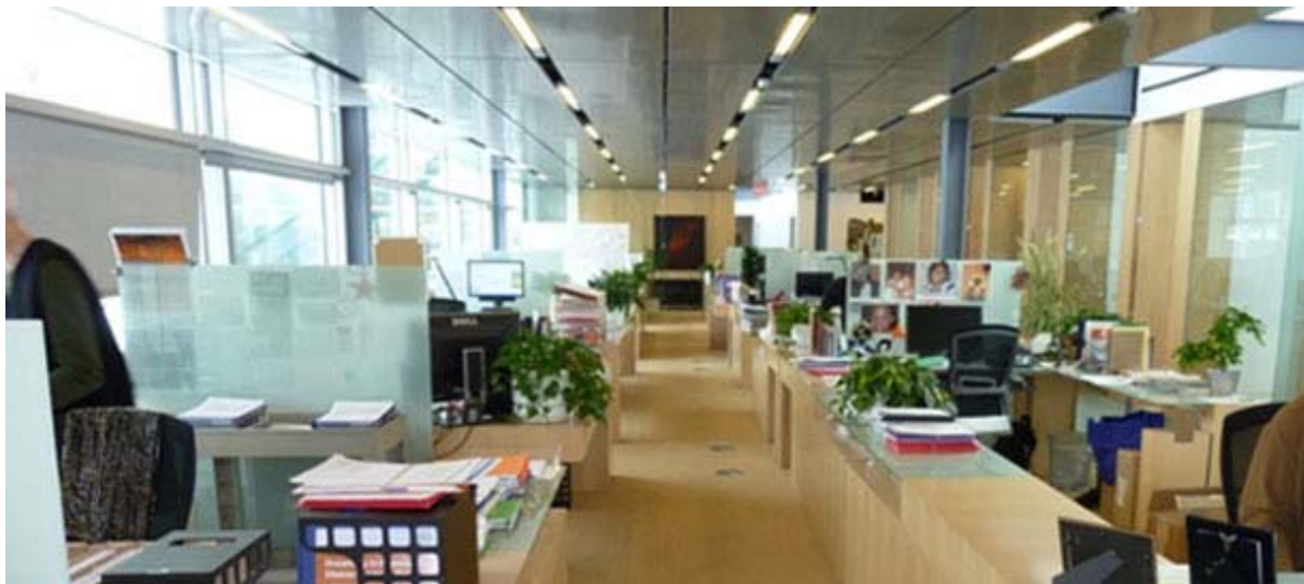
Figure 12: Southern open office area on first floor with ample daylighting but with all light fixtures turned on
